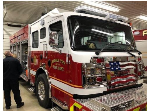
The Radnor Township Fire Department has recently put into service a 2022 Rosenbauer Fire/Rescue vehicle. The new engine is equipped with a 1,750 gallon per minute pump, hydraulic rescue tools, 4 person cab, miscellaneous fire / rescue tools, light tower, and green electric generator. The truck is designed to respond on auto accidents, miscellaneous service runs, and fire runs (as second engine). The Rosenbauer replaced our 1999 FireMaster Engine/Rescue.
